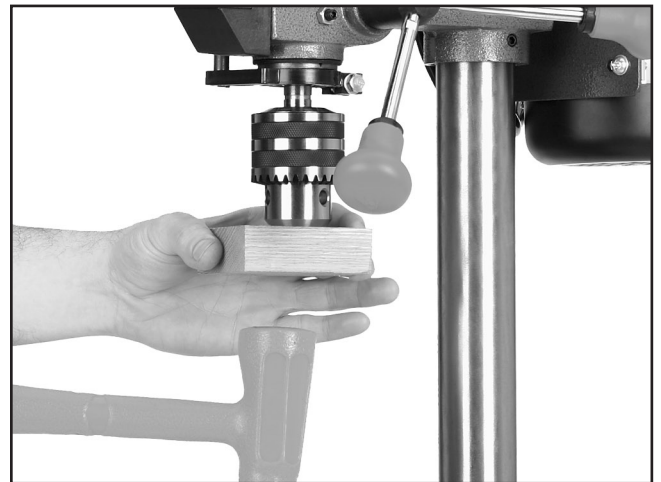
Figure 10. Seating the chuck on the spindle.
